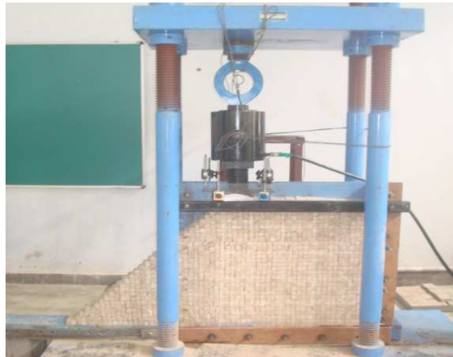
Figure 2: Bearing Capacity Test Apparatus (J0090SL45)
