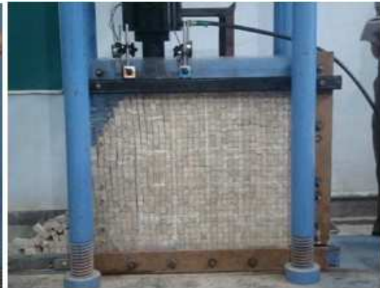
Figure 4: At Failure for the Test J0090SL90 Figure 5: At Failure for the Test J0090SL75
